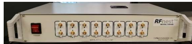
IAI's RFnest: network channel emulator (adds pathloss, fading, Doppler, multipath effects to RF signals)
